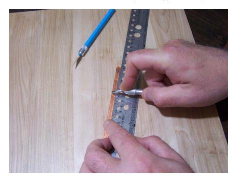
3. Make only a single line of rivets at each of the outer edges. The outer edges will rest adjacent to another 6-inch length of tape on both sides. You are now finished with the first strip of copper tape. You can make as many as you can. They will look like this:
