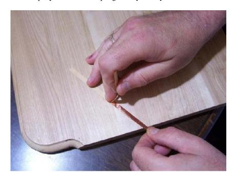
7. The best place to install the first strip of copper is at the stern-most edge of the bottom of the keel. So, using both hands, attach the copper strip there. Make sure it is centered, even, and has no wrinkles. It can still be lifted with an X-Acto knife to make adjustments at this point. Once you are satisfied, press it down
