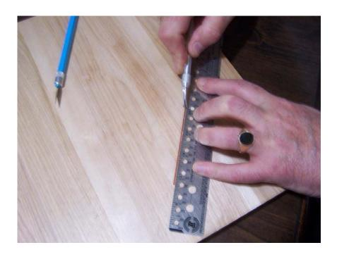
2. Now take the strip of copper and place it against the outer edge of the steel ruler. Using the pounce wheel, make double lines at 1-inch intervals to represent the riveted separations between plates. Mark these perpendicular and between the upper and lower lines of rivets. Start at the top of the upper rivet line and go down to the lower rivet line, with the steel ruler acting as a stopper for the pounce wheel.
